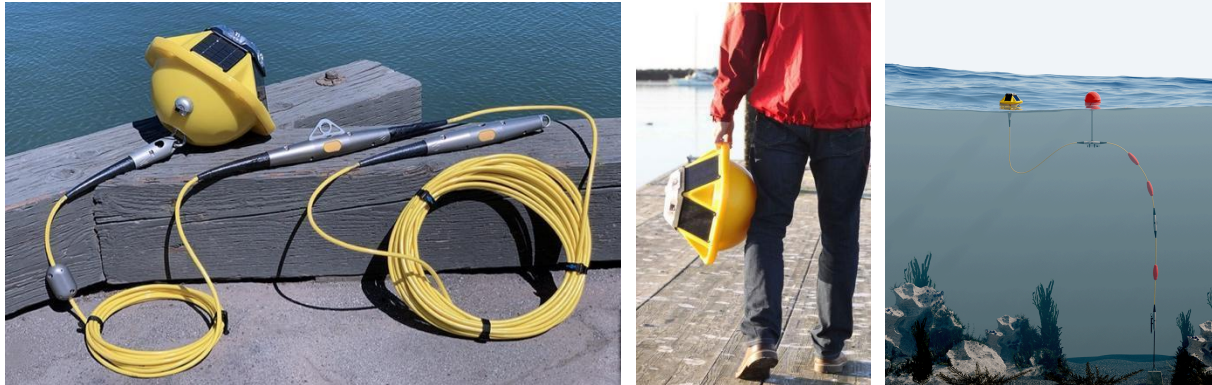
Figure 1. Spotter with Typical Smart Mooring Configuration
