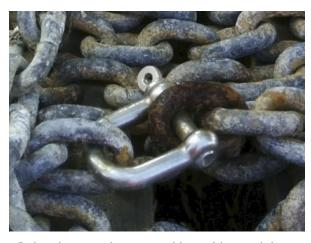
Galvanic corrosion caused by pairing stainless steel with galvanized chain. More info can be found on this helpful rigging website.
